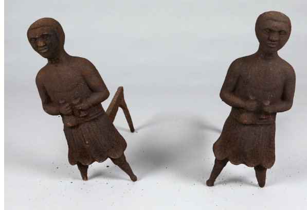
ABOVE Andirons before treatment, unstable and actively corroding. LEFT Andirons after treatment, including restored legs and carbon fiber mount.
