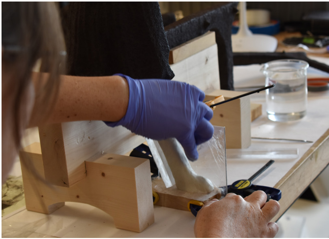
LEFT Sculpting new legs with epoxy, using clamps and plastic backing as temporary support. BELOW Carbon fiber mount, which fits under the skirt and down the legs to the feet for support of the heavy weight.
